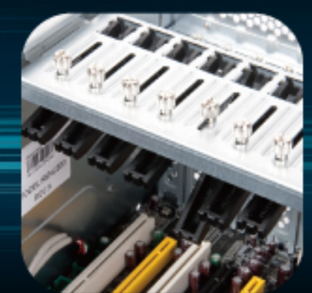
Screwless adjustable card retainer for standard or low profile card
